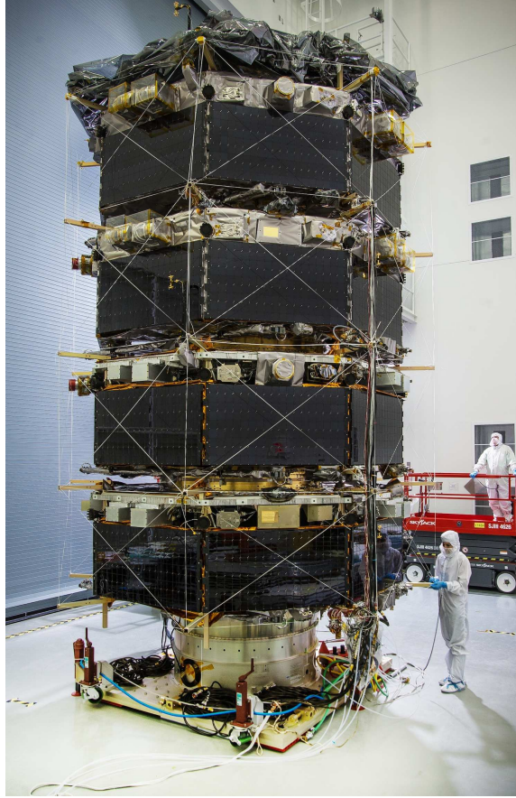
Figure 1.1: Photograph of the MMS Observatories in their stacked configuration for launch. Each Observatory is identical. (Image from [1])
